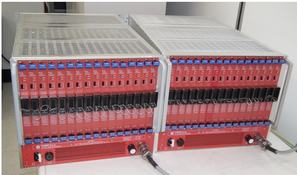
CAEN mainframes hvcaentest2 and hvcaentest3 in EEL 121b. Each are fully populated with sixteen A7030TN HV cards.
